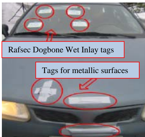
Photograph 3: Tags on the test car and their location
